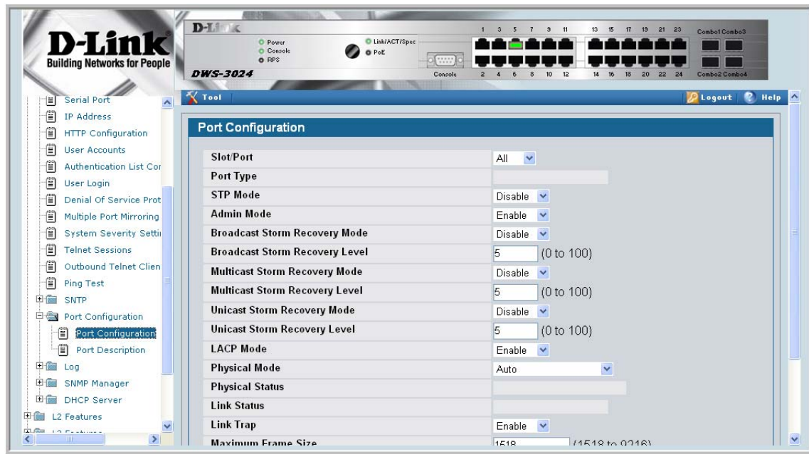
Figure 8. Port Configuration (Storm Control)
