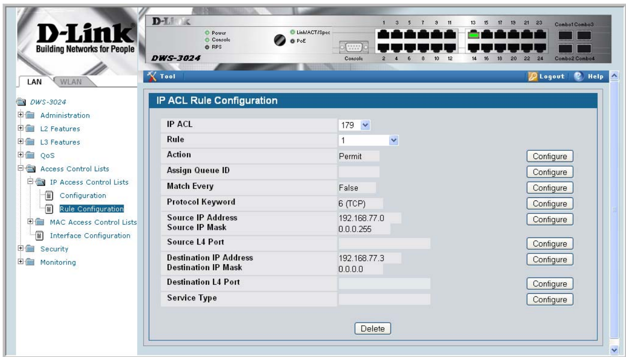
Figure 57. IP ACL Rule Configuration Page - Rule with Protocol and Source IP Configuration
